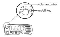
When the radio is first turned on, the red, green, and amber LEDs flash briefly and the radio gives two short beeps. A brief message may appear on the display.
